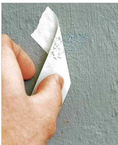
Result of cross-cut adhesion test on concrete surface. Lots of particles torn out: substrate only suitable for masking to a limited extent.
